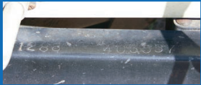
Coachmen serial number at rear cross member, passenger side. 1288 403557
