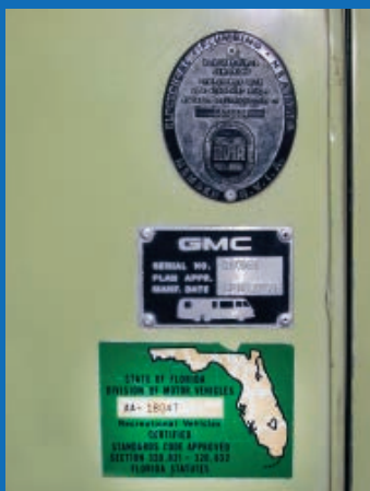
RVIA badge on all RVs, GMC plate on about 20% of GMC Motorhomes, state decal applied as required.
